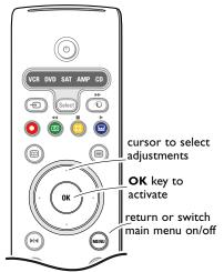
Press the MENU key on the remote control to summon the main menu. At any moment you can exit the menu by pressing the MENU key again.
